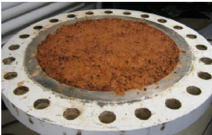
Figure 2b: soil from the site on top of geomembrane in the test cell
